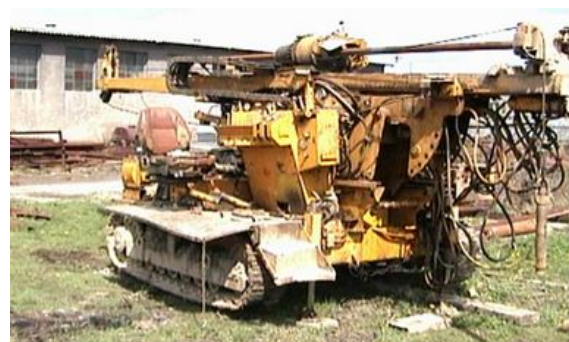
Obr. 46: Vrtná souprava DIAMEC 250 [12]
