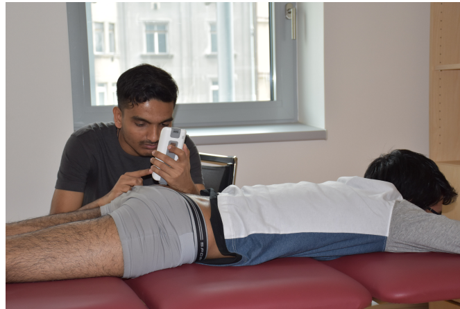
Figure 3.6: Measurement of the parameters from Gluteus Maximus(GM) Muscle by using MyotonPro device.
