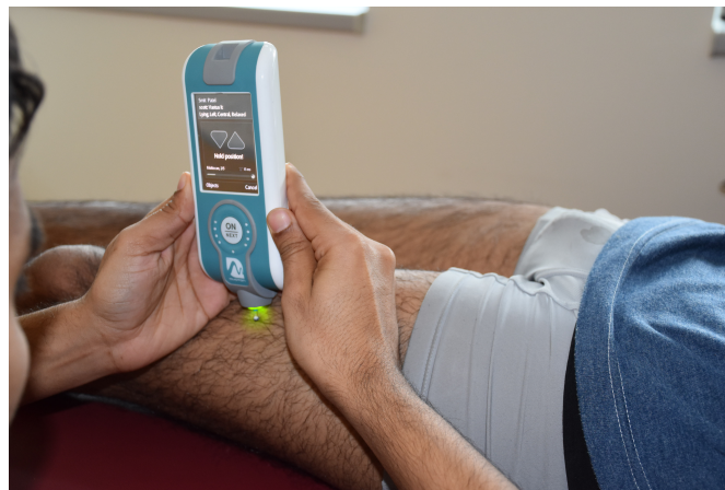
Figure 3.7: Measurement of the parameters from Vastus Medialis(VM) Muscle by using MyotonPro device.
