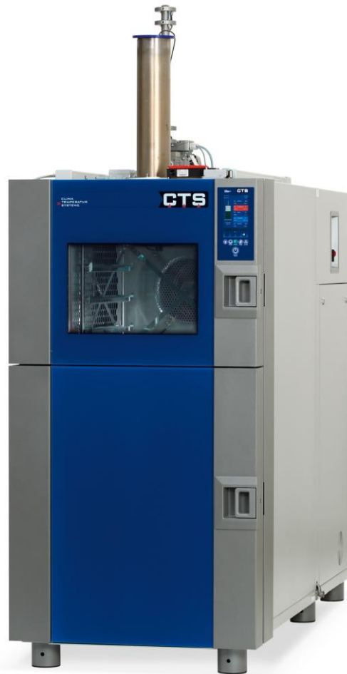
Figure 14. Thermal Shock Test chamber (TSS series) used for stress testing our ECA samples [38]
