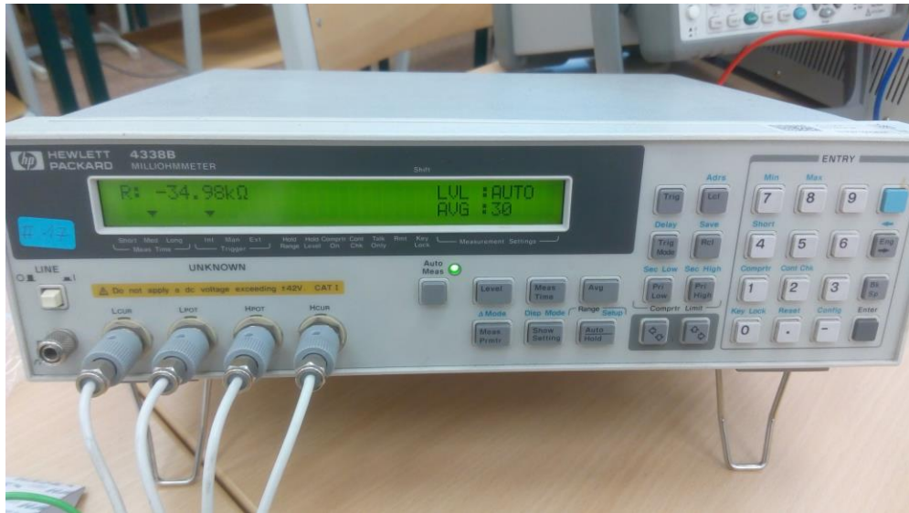
Figure 13. Milliohm meter Agilent HP 4338B used for resistance measurements
