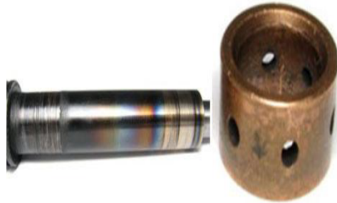
(b) Shaft and bearing wear caused by lack of lubrication supply. Blue discoloring results from over-heating of the shaft due to metal-to-metal contact. Figure adopted from Polichronis et al. (2013).
