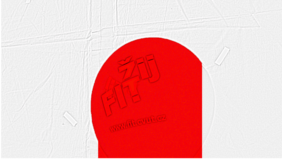
Figure 4.3: An object found by Boykov-Kolmogorov algorithm from the image in the Figure 4.1.
