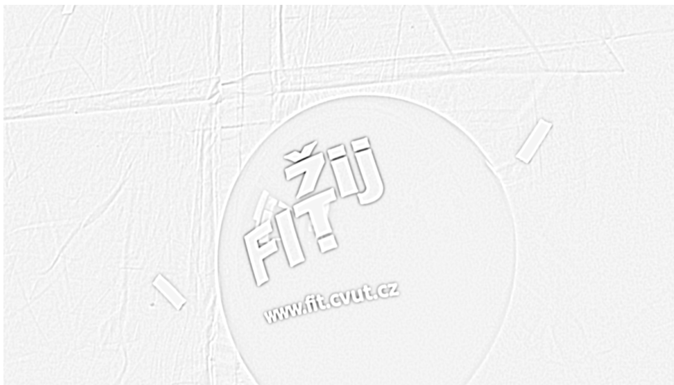
Figure 4.2: Image after Laplacian of Gaussian filter was applied.
