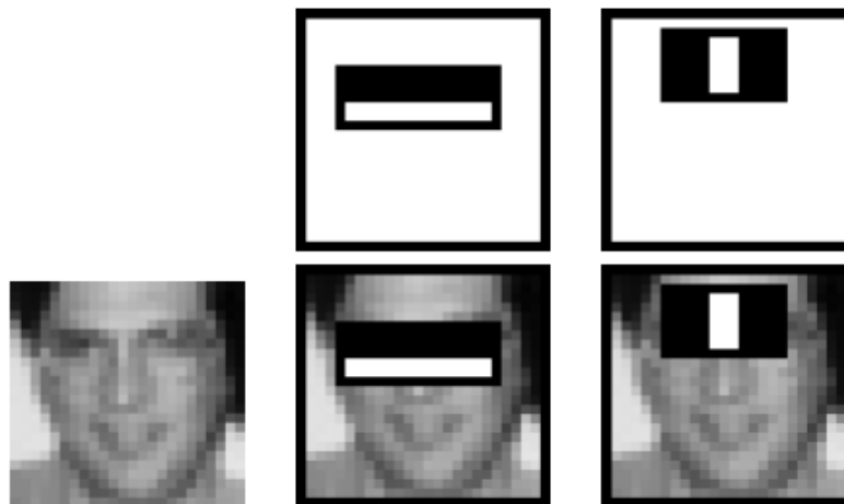
Figure 7: Haar-like features selection in Viola-Jones framework. The figure presents the work of the AdaBoost framework [43]. The features are chosen based on the intensity of the selected region. The first selected features (row no. 2, second image) are differentiating eyes from the rest of the face. The second feature (row no. 2, third image) distinguishes between the eyes and the nose bridge.
