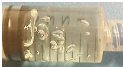
Figure 34: Large air inclusions in coupling medium stored in a syringe
