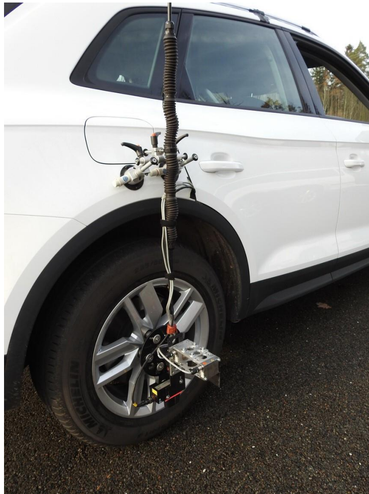
Figure 21 - Displacement sensor mounted on the vehicle
