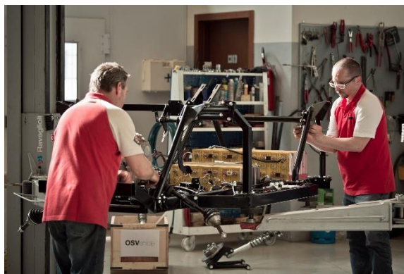
Figure 16 Assembling of TABBY EVO platform lasts one hour and demands only two workers
