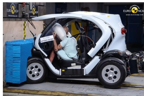
Figure 7 Renault Twizy. Full-width frontal impact
