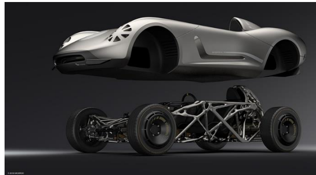
Figure 12 Space frame of company Hackord is built by 3d printing
