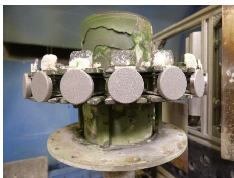
Pic. 15 Support head with the T91 steel specimens prepared for plasma coating
