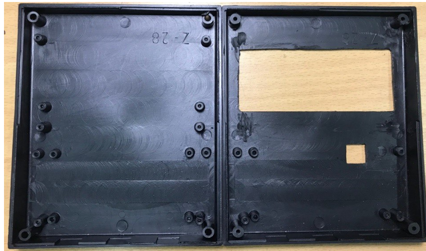
Figure 3.11. Plastic cover with drilled openings.
