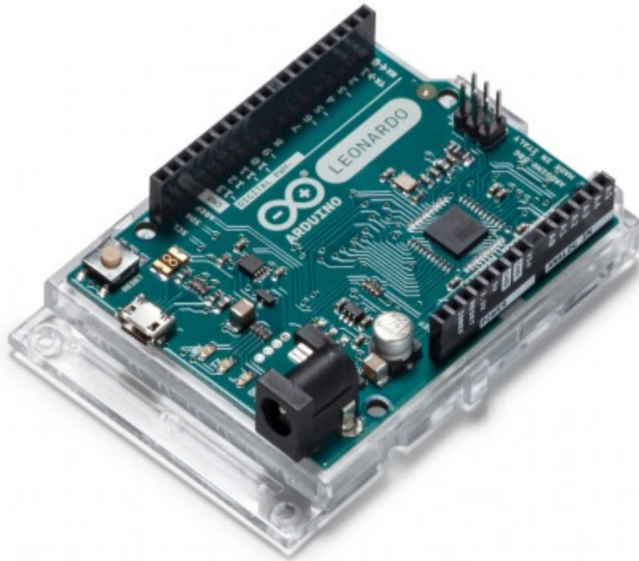
Figure 3.1. Arduino Leonardo microcontroller [9]
