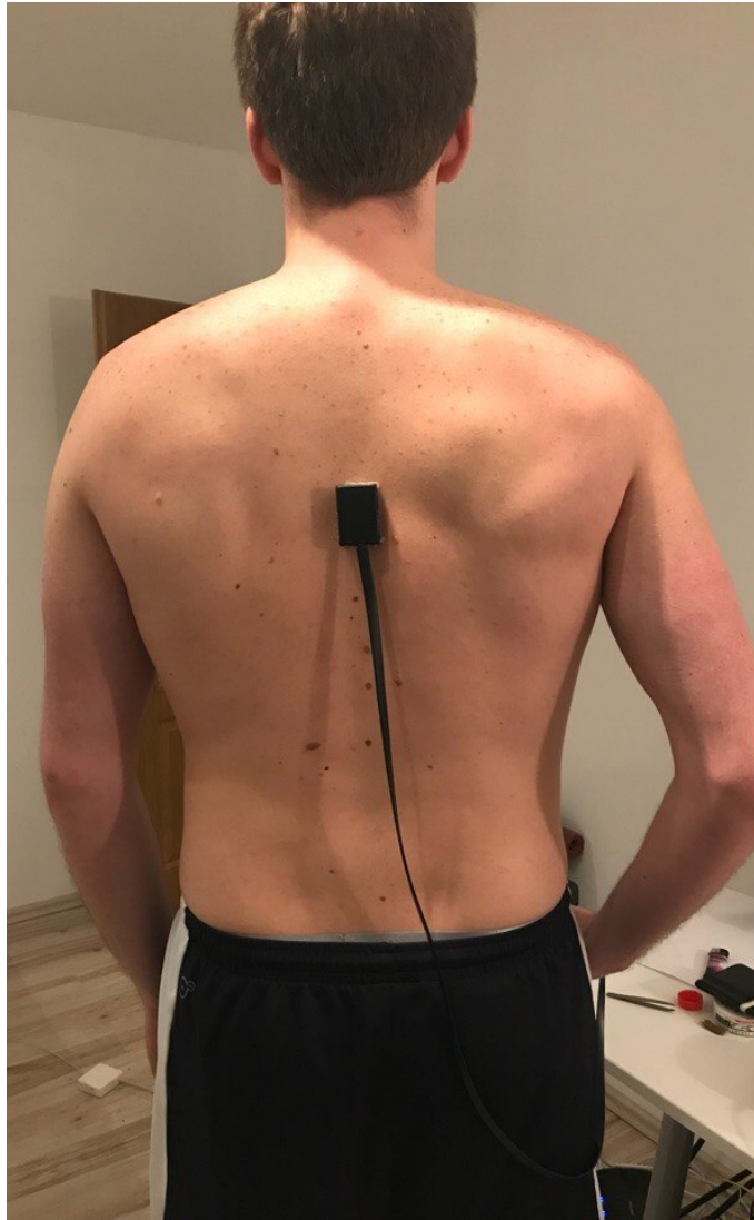
Figure 5.7. Positioning of sensor on upper back between the shoulder blades
