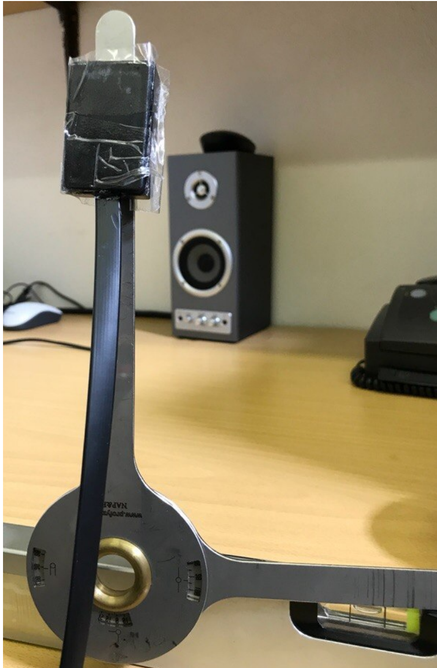
Figure 5.4. Verification of calibration of z(\text{yaw}) angle using a protractor and level
