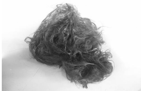
Fig. 1. Recycled CF from aircraft components.
