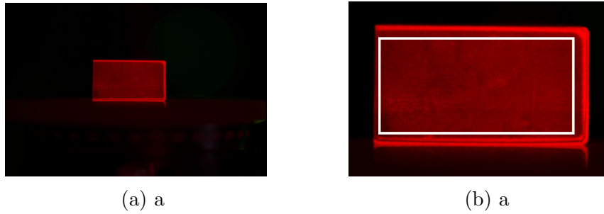
Figure 5.3: The image acquired by the camera (a) and the cropped picture of the sample. The white rectangle is the selected area of the crystal (b).
