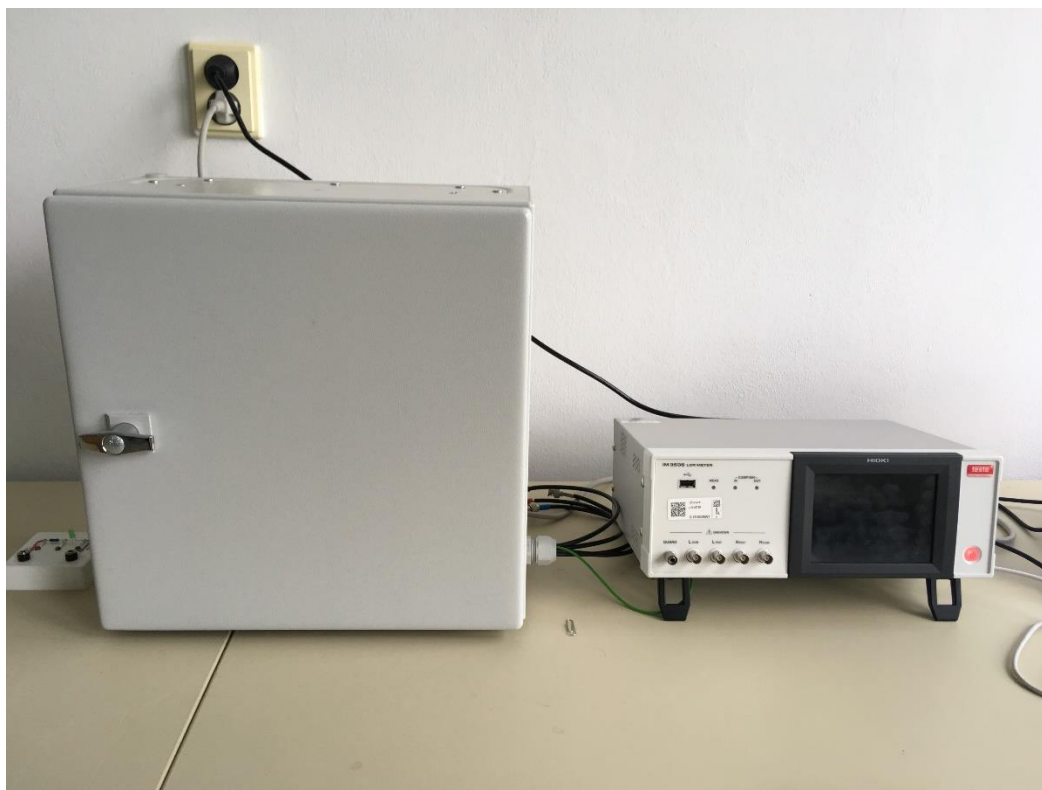
Fig 16. Chamber (left) for the measurement impedance with LCR Meter (right).
