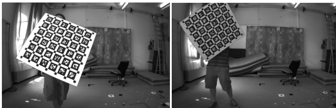
Figure 2.4: A typical calibration of a stereo camera system’s external and internal parameters. The procedure requires a lengthy process of acquiring images of a large planar pattern. The images need to be synchronized in time. Image courtesy of [13].
