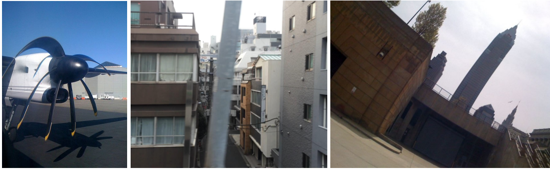
Figure 1.1: Examples of rolling shutter induced image distortions. A fast moving object in a still shot (left), courtesy of Soren Ragsdale. Translational motion of the camera (center) and rotational motion of the camera (right), courtesy of Greg Kopec. In this thesis we will deal with the cases such as the two examples from the right.
