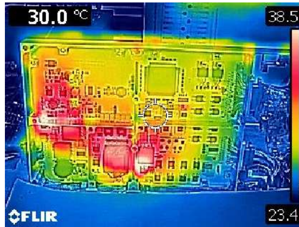
Fig. 58 RPWI LVPS EM2 Thermal Footprint under full load conditions.
