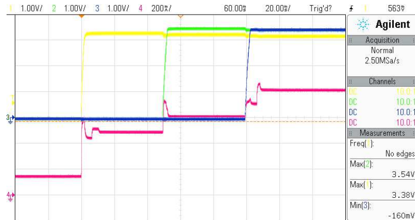
Fig. 79 The input power bus current captured during the sequenced instrument power on with suppressed inrush current spikes by the use of Digital Inrush Current Limiter, [SP-1].
