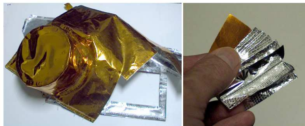
Fig. 1 Multilayer Insulation example as a protective layer for spacecraft sensor (left), the composition of temperature insulating layers of the MLI (right), [I-1].
