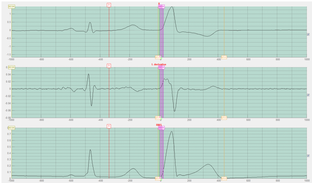
Figure 4.5: Allocation of the final PVC onset (green line) set by the algorithm and six time markers (pink lines) defining sub-intervals of the selected initial 30 ms time interval. Orange lines mark selected baseline time markers IZO1 and IZO2 . Upper graph: standard lead II. Middle graph: Derivative of the lead II. Lower graph: RMS signal computed from all measured chest leads
