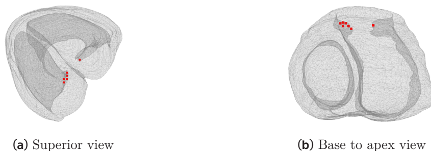
(a) Superior view (b) Base to apex view Figure D.11: Positions of the twenty-five dipoles of the inverse solution with minimal RRE. Inverse solution was solved using the combination of homogeneous torso model H and TIBSPMs computed for 8 ms. Five dipoles (instead of one) with minimal RRE were selected for each inverse solution for 5 PVCs (see sec. 3.5.7 and 5.6.2) for Pat004
