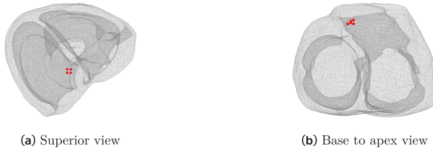
(a) Superior view (b) Base to apex view Figure G.12: Positions of first five dipoles with minimal RRE value of the inverse solution for one BSP map (IBSPM 0–15 ms) and homogeneous torso model H (see sec. 3.5.7 and 5.6.3) for Pat007
