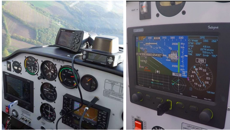
Figure 10.18: Aircraft pilot panel with the integrated Safely system—build-in EFIS Integra, Zaon PCAS with the GPS on the flight panel. Rest of the system is integrated under the panel.
