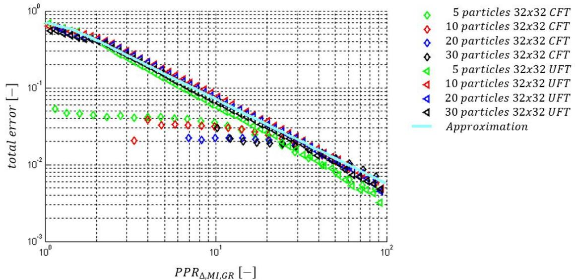
FIGURE 5. Dependency of the corrected metric  $PPR_{\Delta,MI,GR}$  on the total error of the measurement. Results of synthetic tests UFT and CFT for four different numbers of the particles. Velocity gradient inside IA was between the values 0 to 1.5.
