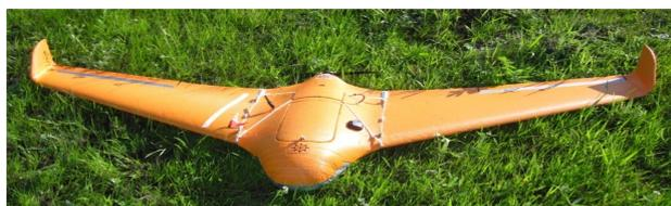
FIGURE 2. SX8FW (with the mini autopilot developed in at the National Aerospace University (KhAI)).
