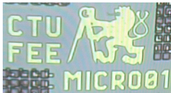
Fig. 4.14: One of the smallest emblems of the Czech Technical University in Prague with the width of 59.55 μm and the height of 44.85 μm is present on the fabricated chip
