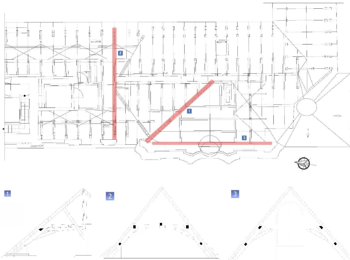
Figure 4.1 – Base plan drawing of the southern part of the west wing roof (top), Frame 1 (left), Frame 2 (center) and Frame 3 (right)
