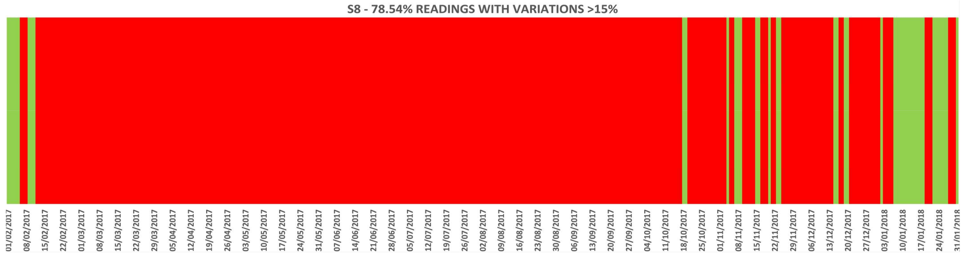
Figure 33 - Sensor 8. Time line with all the readings along the year with variations higher and smaller than 15% in terms of Relative humidity (RH). Green <15%; Red >15%.
