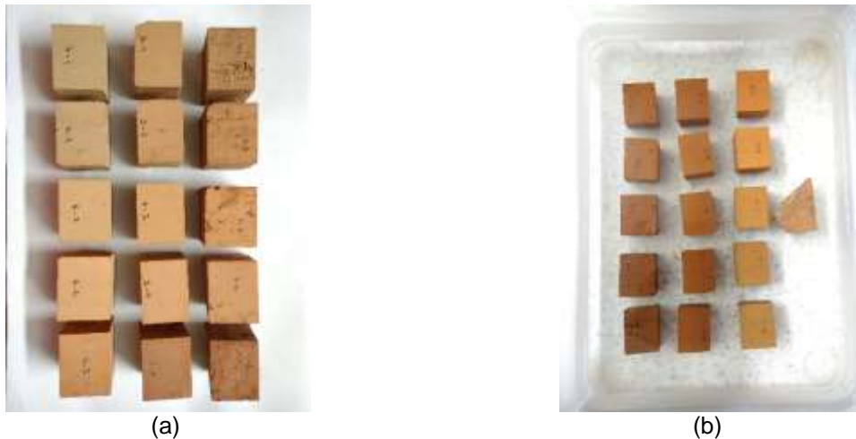
Figure 25- Water absorption test; (a) dry specimens; (b) specimens saturated in distilled water.
