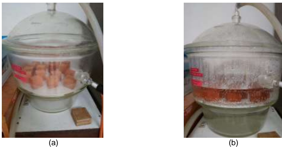
Figure 26- Porosity test; (a) Specimens placed under vacuum; (b) specimens placed under vacuum in saturated condition.
