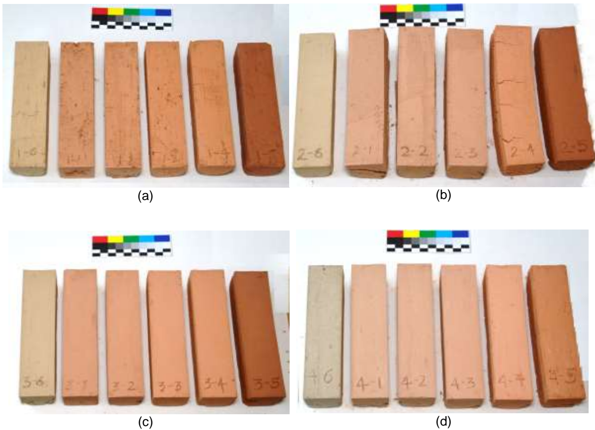
Figure 22- Display of burnt ceramic specimens for each clay sample burnt at different temperatures; (a) Specimens of clay sample 1; (b) Specimens of clay sample 2; (c) Specimens of clay sample 3; (d) Specimens of clay sample 4.
