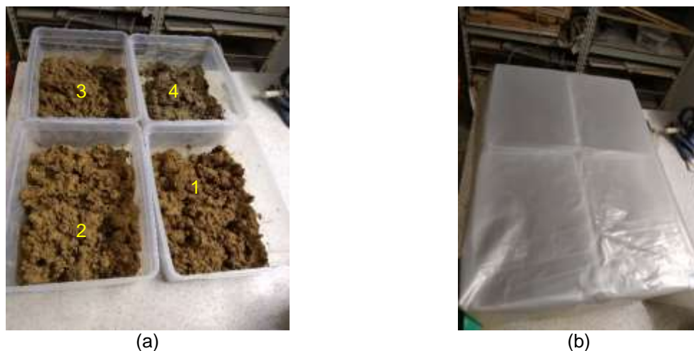
Figure 18- (a) Final addition of water to the samples; (b) Covering the mixture with plastic in order to prevent evaporation.
