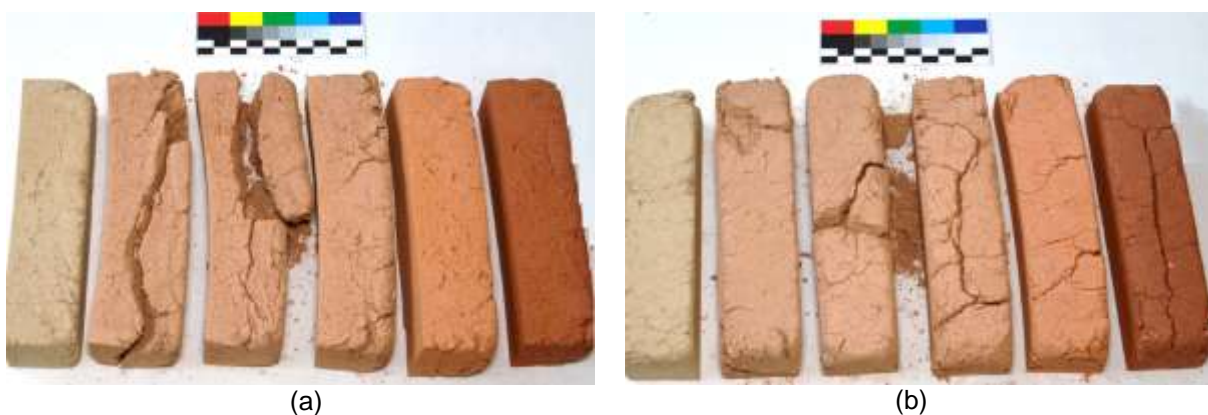
Figure 23- Spalled and cracked specimens of clay sample 2; (a) Side profile; (b) Back profile.
