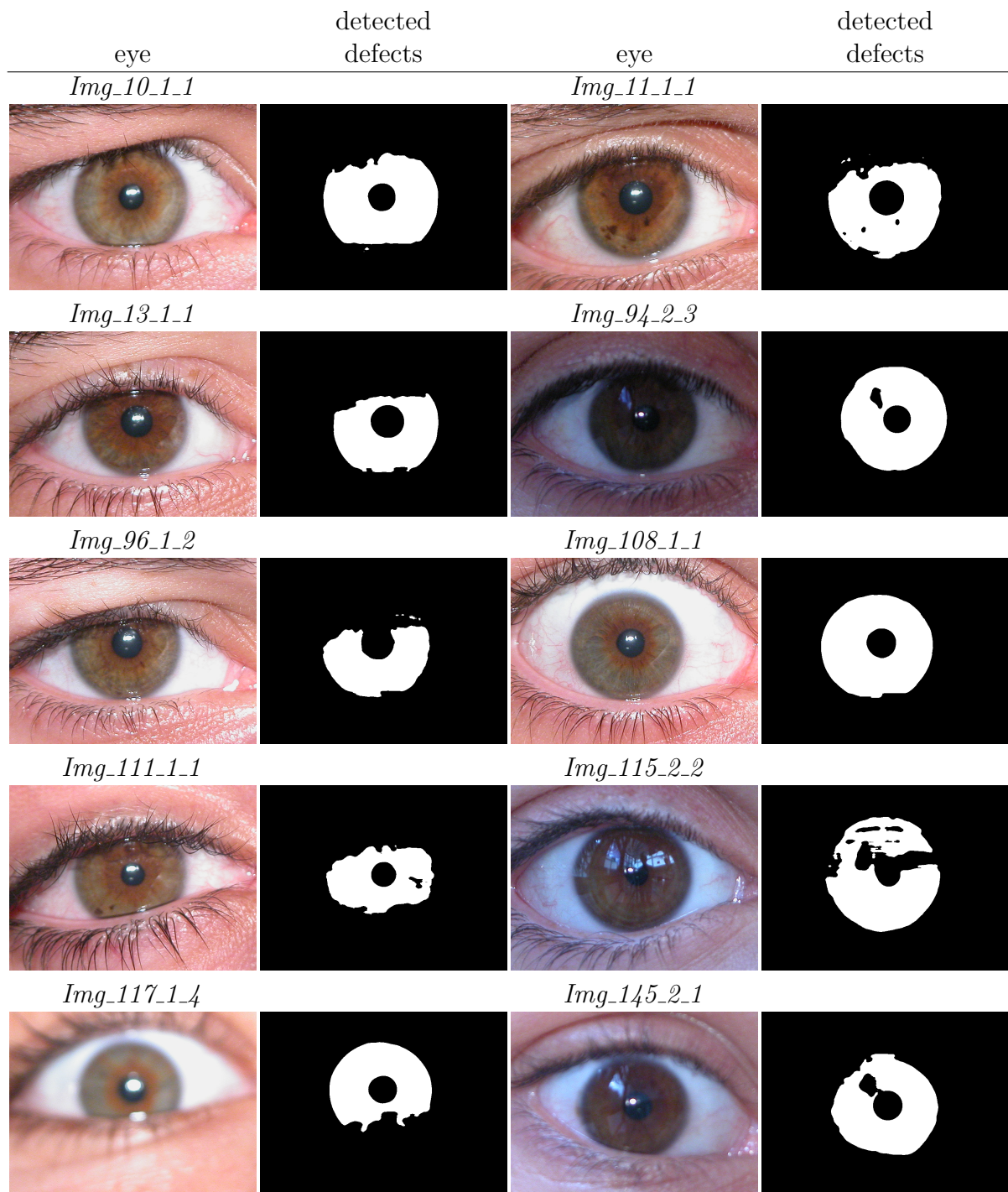
Figure 7.1: Eye images and the corresponding detected occlusions masks in the first method (UBIRIS database). Above the iris image in odd column is name of the iris in database. For numerical results of selected irises see Table 7.1.
