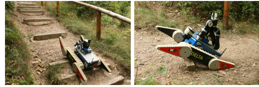
Fig. 13. Climbing an 70-meters-long exterior staircase with our robotic platform. It was additionally equipped with a robotic arm (right image) to test different weight distribution effect on the trajectory estimate and model robustness.
