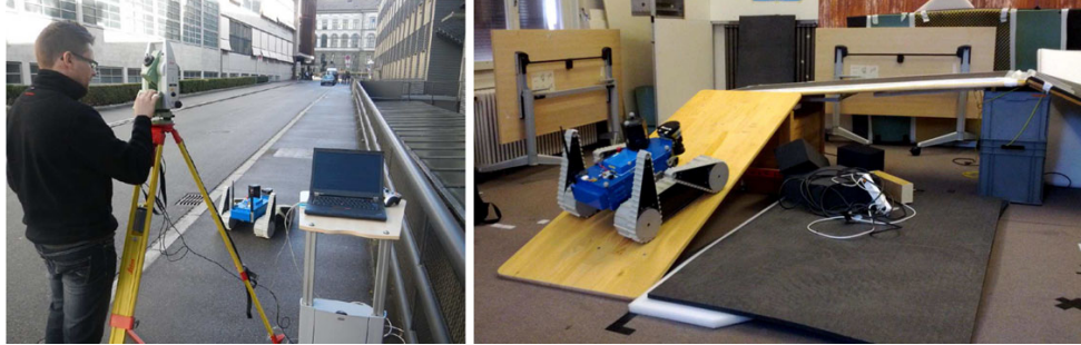
Figure 5. The experimental setup with the Leica reference theodolite for obtaining ground truth trajectory (left). Part of the 3D semistructured environment for an indoor test with motion capture ground truth (right).
