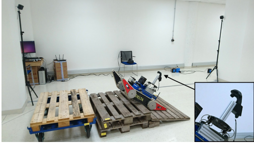
Fig. 7. Indoor experiment with HTC Vive reference system. Detail shows a HTC Vive controller attached to the robot via vibration dampener, which is necessary due to an IMU inside the tracked controller.
