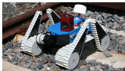
Fig. 1. Skid-steer mobile robot (the UGV) for search and rescue operations developed by BlueBotics (www.bluebotics.com) as part of NIFTi project.
