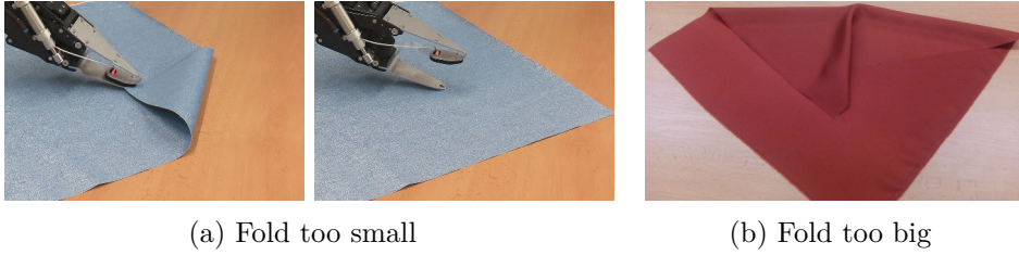
Figure 8.7: Scenarios in which the folding is not possible. In the scenario (a), the folded state is not stable. After the gripper releases the garment, the garment returns into the spread state. The scenario (b) shows the collapsed state of the garment. It occurs when the garment edge measured between the gripper and the desk is too long. The forces acting on the garment cause that the edge moves towards the grasping point although the gripper remains static. It results in the collapsed state at the end.
