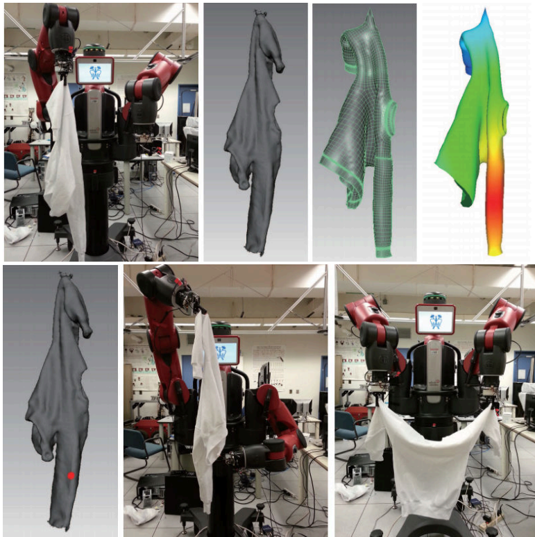
Figure 2.4: The unfolding of the hoodie with a baxter robot. The top row shows from left to right: the robot grasping the garment, reconstructed model, model matched in simulation, and the predicted mesh with Gaussian distribution distance. The bottom row shows from left to right: the predicted second grasping point, the regrasping step, and finally the unfolded garment. Images are from [Li et al., 2015a].
