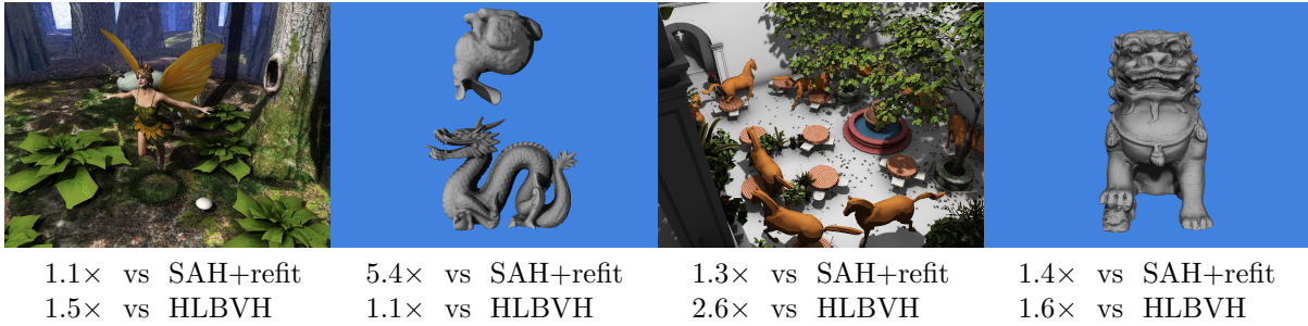
Figure 3.2: Average speedups of ray tracing for several tested animations using our single T-SAH optimized BVH with refitting compared to the SAH with refitting and per-frame reconstruction using HLBVH.
