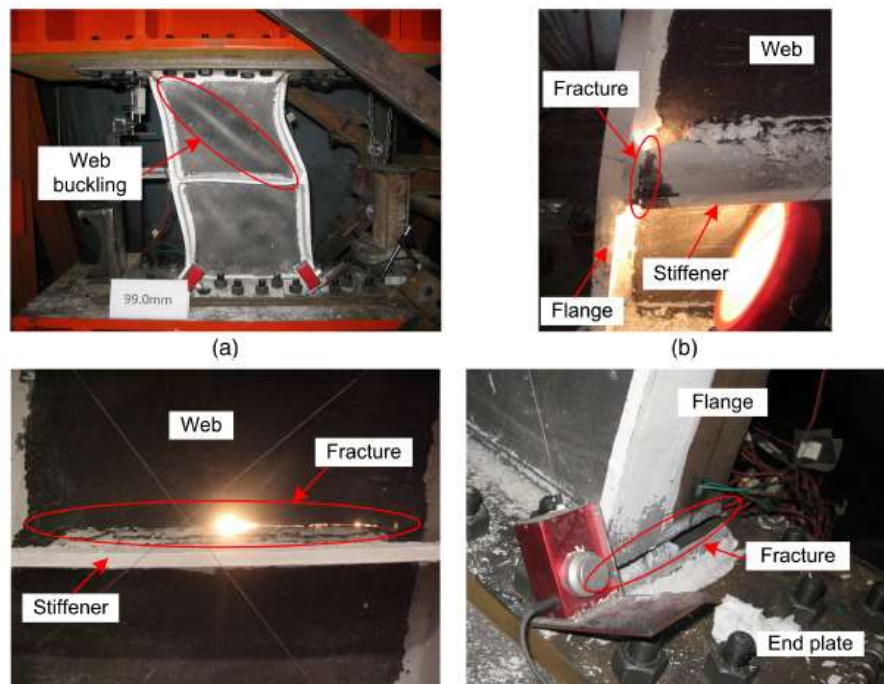
Figure 9. Damage to specimens: (a) web buckling; (b) stiffener-to-flange weld fracture; (c) web fracture; (d) flange-to-end plate weld fracture [14]
