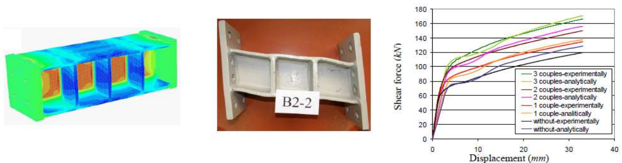
Figure 11. Increase in shear resistance in correlation with web stiffeners
