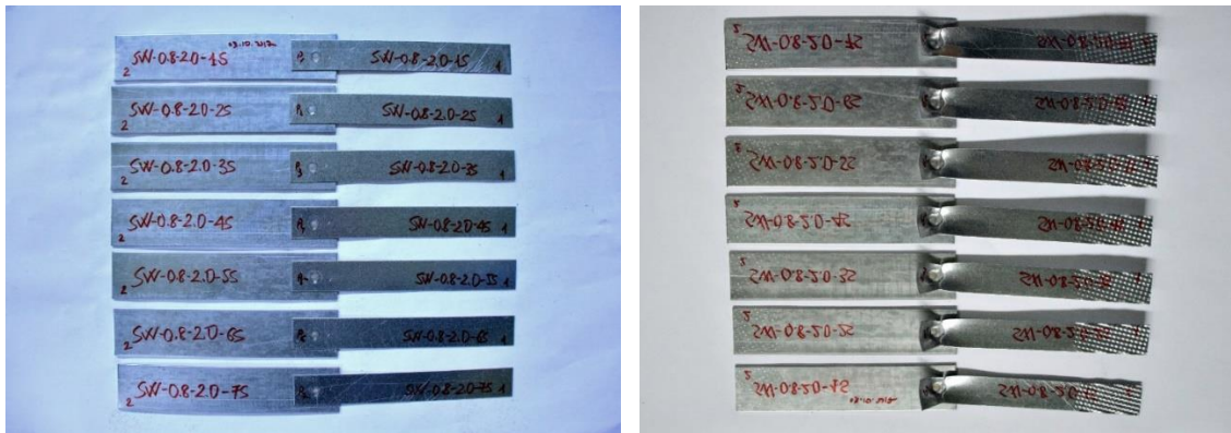
Figure B.6: SW-0.8-2.0 specimens before and after testing
