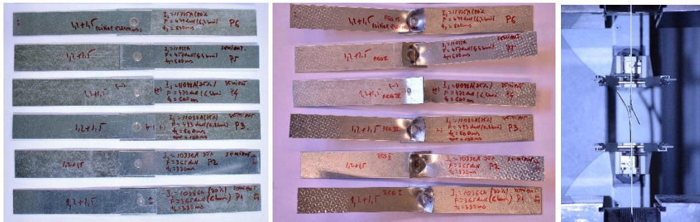
Figure 3.11: Specimens SW-1.2-1.5 before and after testing, using different welding regimes
