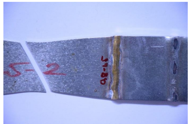
Figure 3.26: Breaking out of heat affected zone
