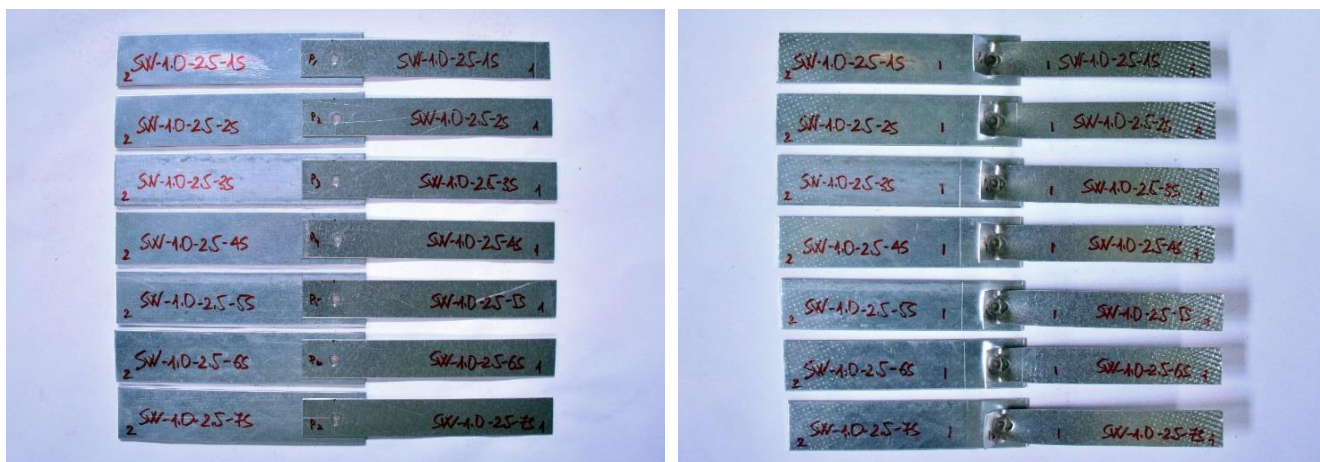
Figure B.8: SW-1.0-2.5 specimens before and after testing
