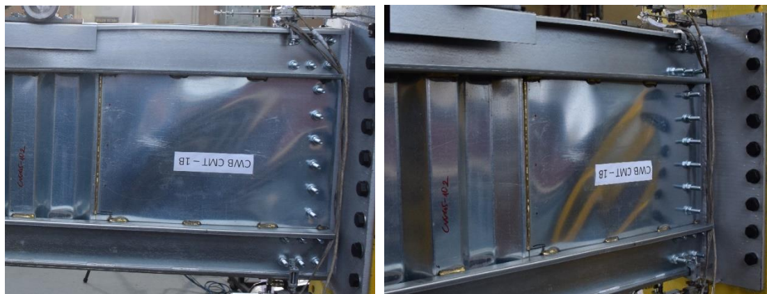
Figure 3.39: Deformed shape of the end shear panel of CWB CMT-1 beam
