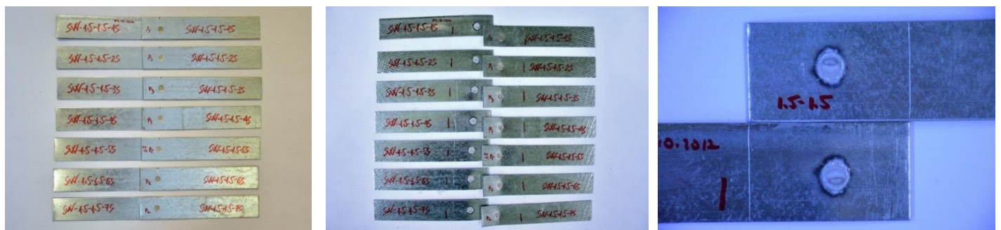
Figure B.12: SW-1.5-1.5 specimens before and after testing and failure mode
