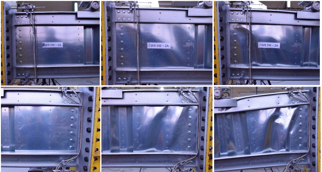
Figure 3.44: Development of the buckling of the end shear panels of CWB SW-2 beam
