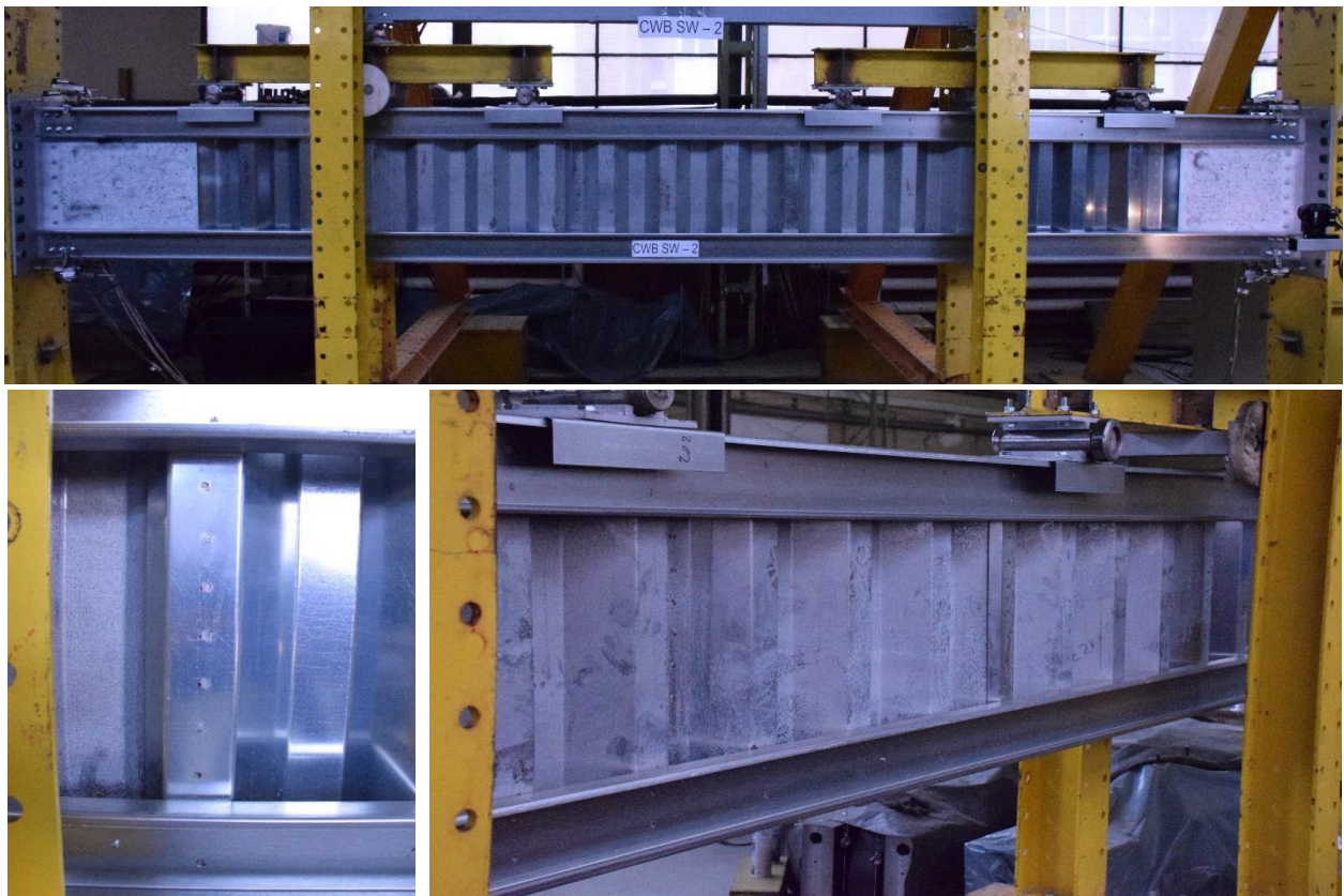
Figure 3.43: CWB SW-2 beam before testing
