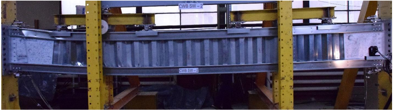
Figure 3.46: Deformed shape of CWB SW-2 beam at failure
