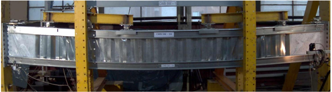
Figure 3.36: Deformed shape of CWB SW-1 beam at failure
