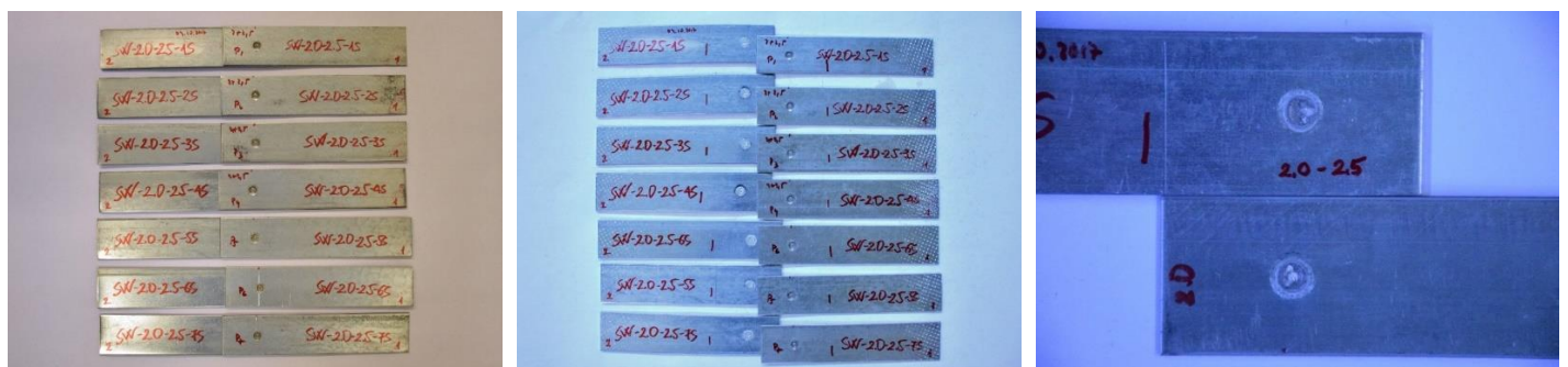
Figure B.13: SW-2.0-2.5 specimens before and after testing and failure mode
