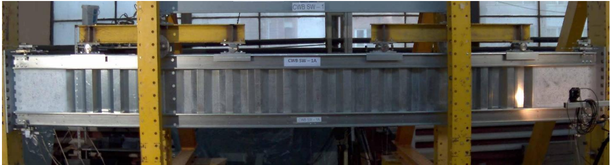
Figure 3.33: CWB SW-1 beam before testing
