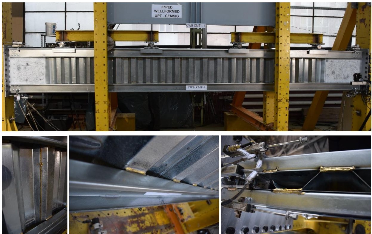
Figure 3.38: CWB CMT-1 beam before testing
