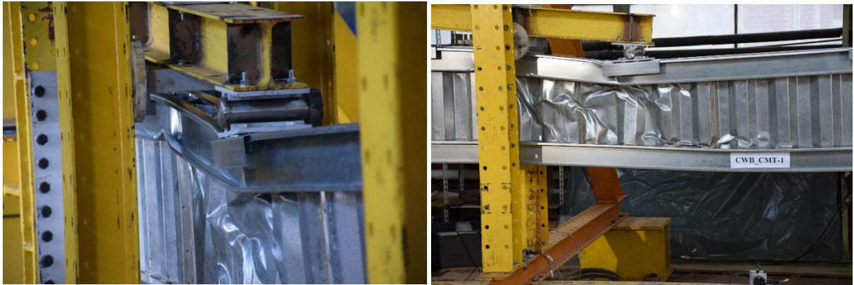
Figure 3.40: Deformed shape of the flange and distortion of the web corrugation of CWB CMT-1 beam
