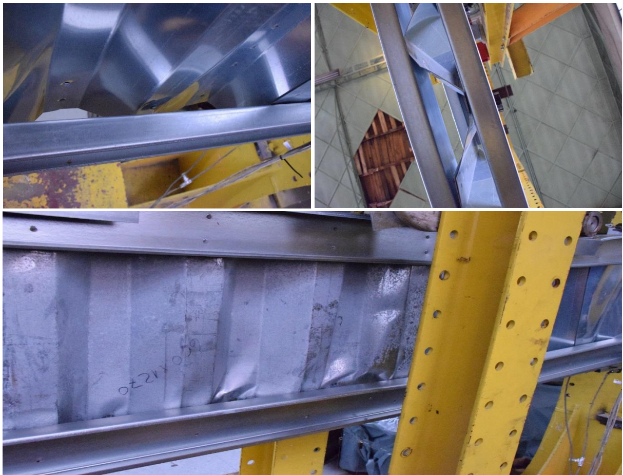
Figure 3.45: Breaking of some spot-welds and distortion of the web corrugation of CWB SW-2 beam
