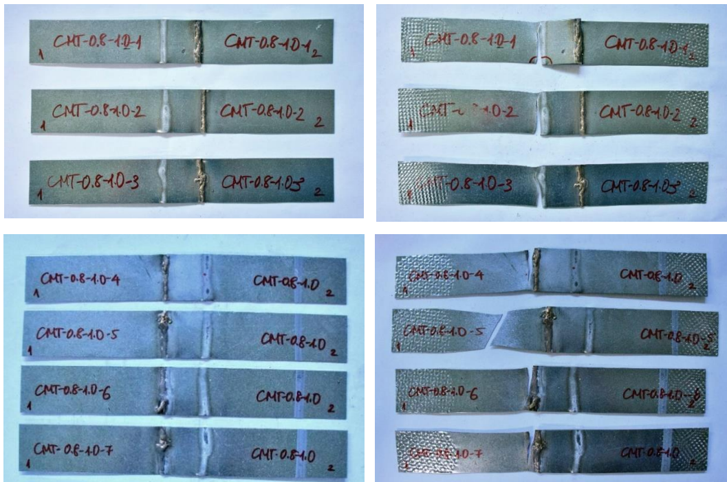
Figure B.19: CMT-0.8-1.0 specimens before and after testing
