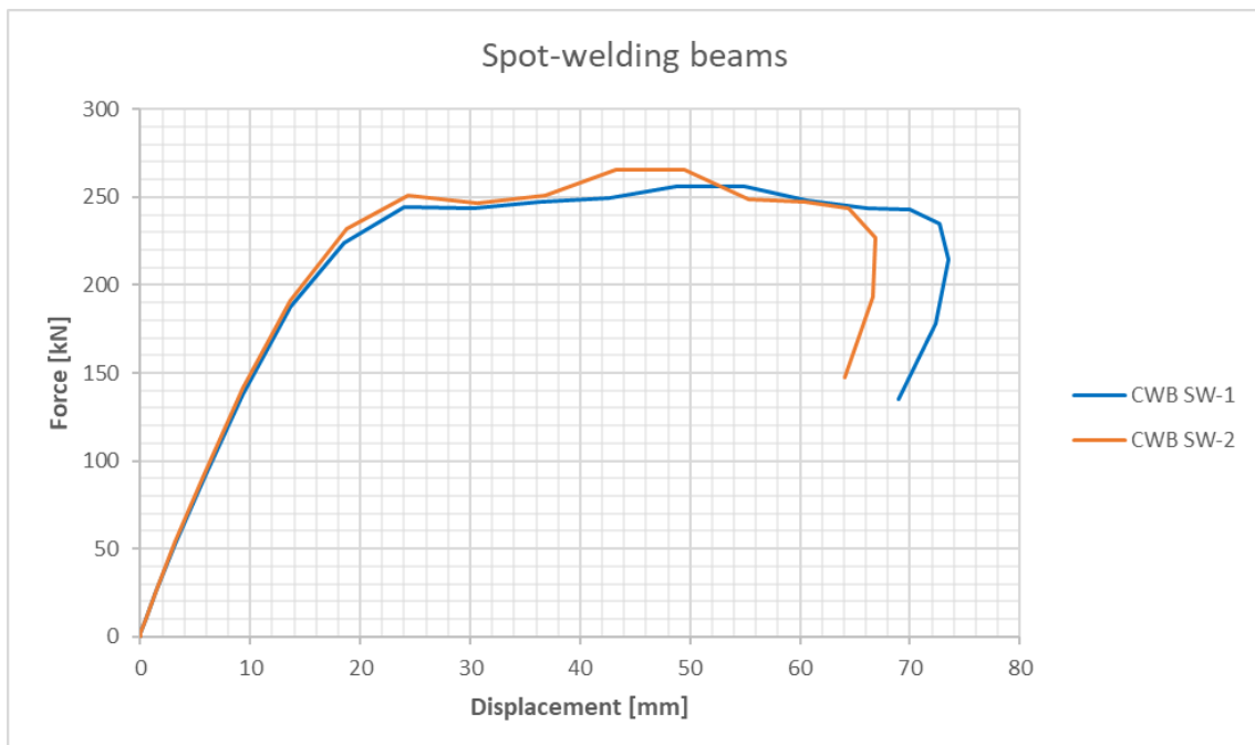
Figure 4.15: Force-displacement curves of SW beams obtained in ABAQUS/CAE
