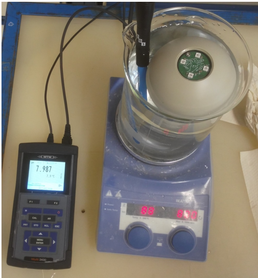
Figure 10 – SQUID during the laboratory testing and calibration. (SQUID is just the ball in the beaker)
