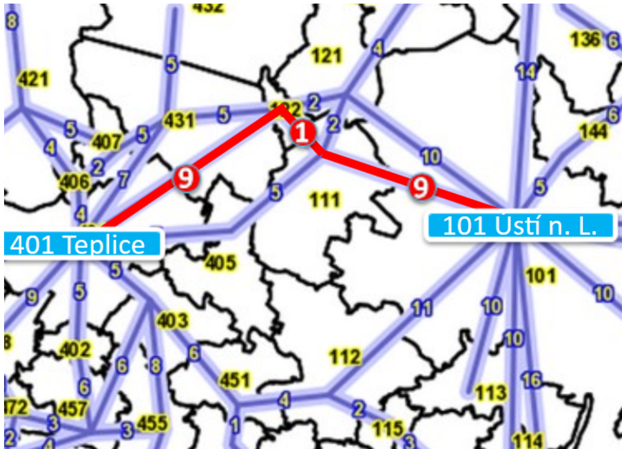
Figure 4.3: Zone-distance tariff in Ústí region. Price is calculated as a sum of distance units between zones in the system. In this example it is 9+1+9=19 distance units that will determine final price.[21]
