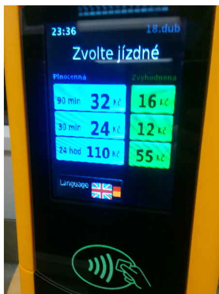
Figure 2.10: Vending machine for on board ticket sale on tram line 18. Only contactless payment cards are accepted. Photo by author.
