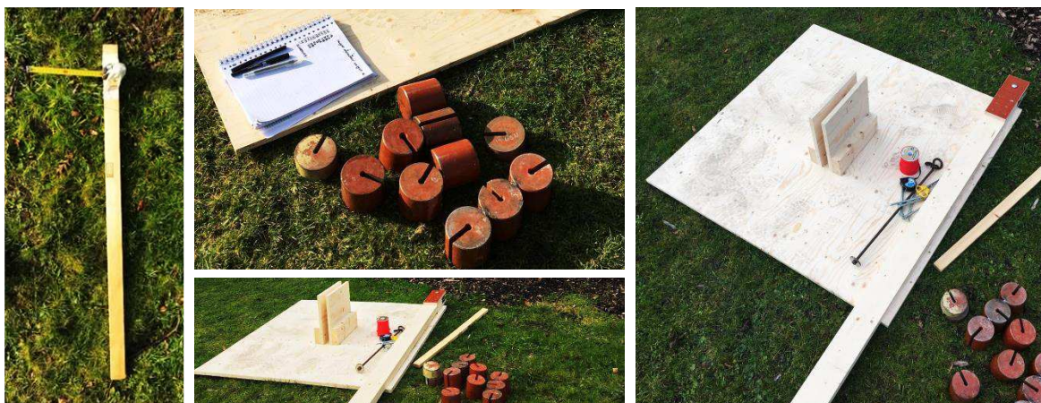
Figure 70. Tools necessary for the pulling test.
