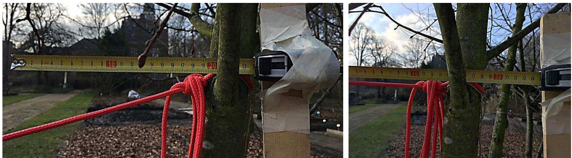
Figure 71. Measuring of the deflection, before and after.
