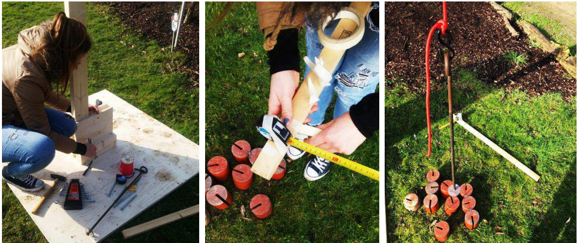
Figure 72. Preparations before the measurement. From left: assembly of the setup after transport, attaching the measuring tape to the lath and preparation of the system of weights.
