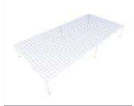
Modelling of a frame - undeformed structure
