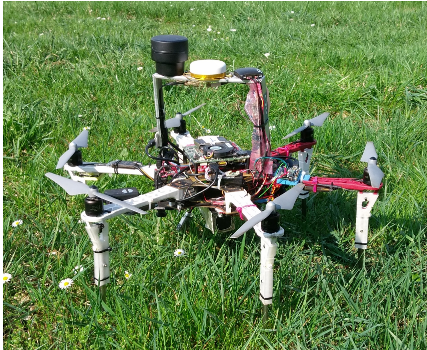
Figure 1: Hexarotor UAV created by MRS research group and used for testing proposed path planning method
