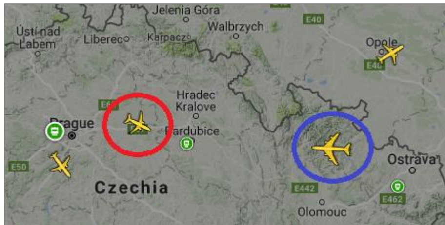
Figure 39 Aircraft situation used for ACAS range determination
