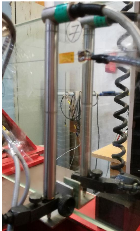
Figure 4.13: 2 rod extensometers placed on a L-shaped steel component
