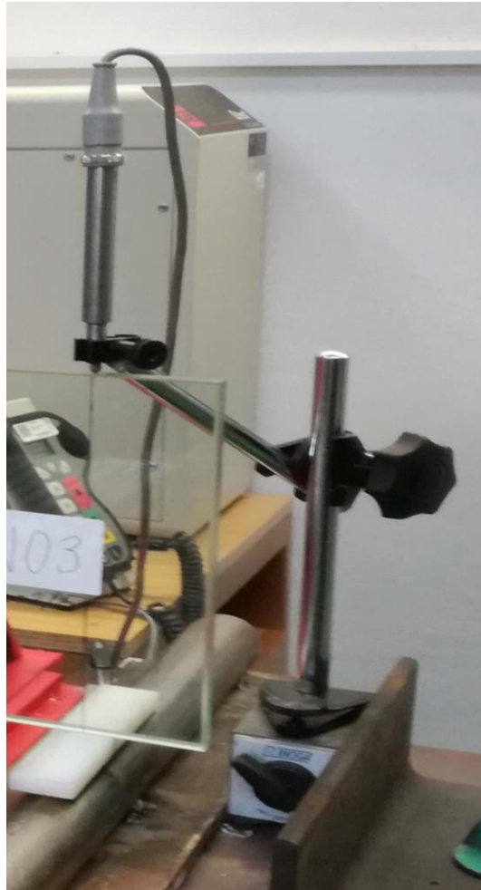
Figure 4.2: Rod-type borehole extensometer with magnetic holder
