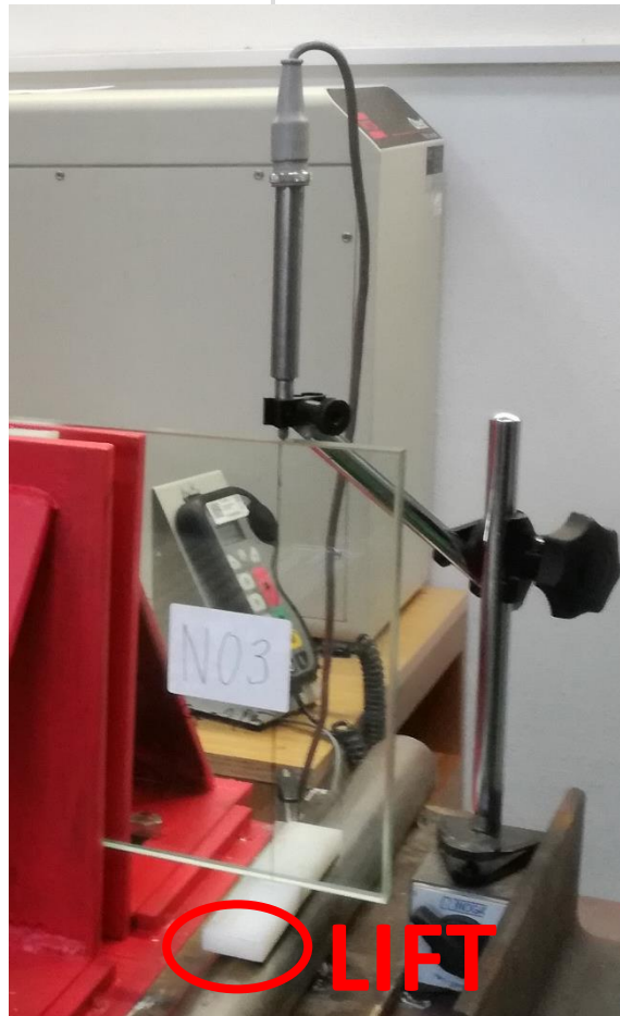
Figure 4.14: Rod extensometer above the support and noticeable pressing of the beam to polyamide
