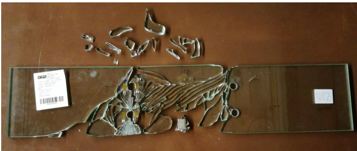
Figure 4.18: The crack pattern of the tested beam
