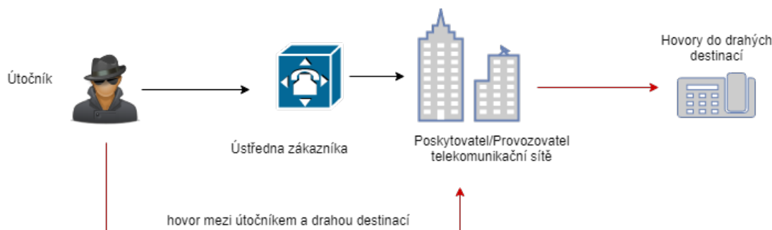
Obr. 2.8: Princip Call Transfer Fraud
