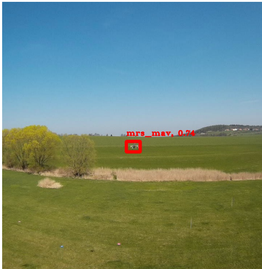
Figure 2: Image from a real-world experiment with MAVs. Output of the object detection convolutional neural network is overlaid in red.
