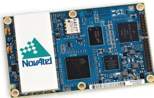
Figure 8.3: Novatel OEM628 GNSS receiver
