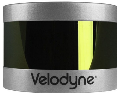
Figure 8.2: LiDAR Velodyne VLP-16
