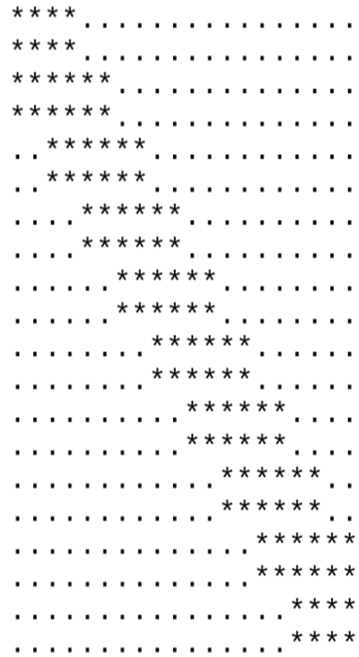
Figure 6.5: An example of a matrix sparsity. [25]. This is a typical look of a matrix, that represents a problem where variables are chained and depend on previous ones.
