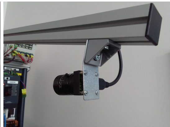
Figure 3.4: Mounting of the camera to the adjustable arm.
