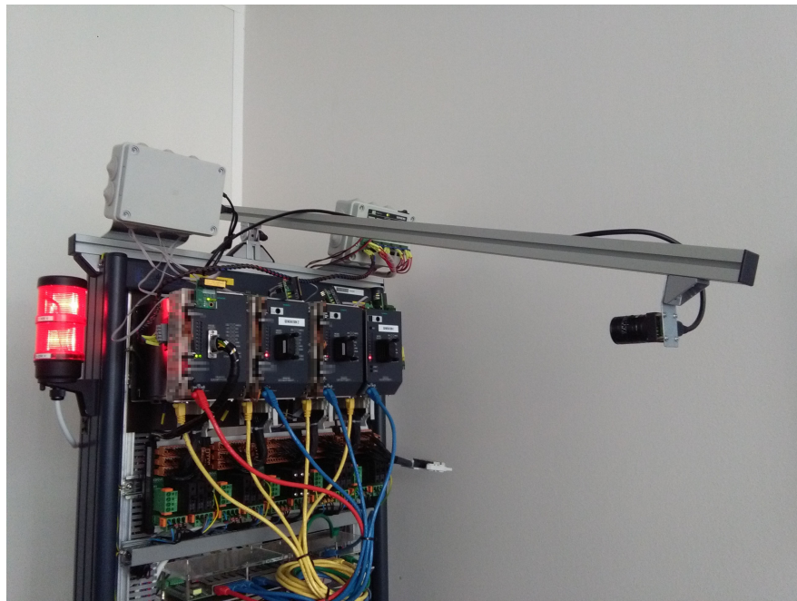
Figure 5.1: Test setup used during testing with attached industrial camera.
