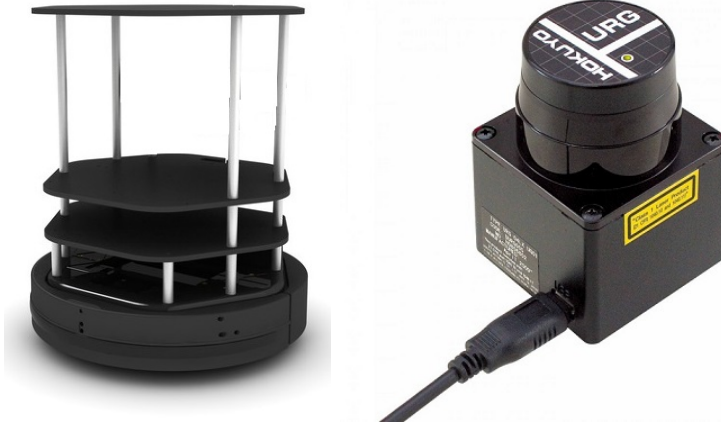
Figure 1.1: TurtleBot and the Hokuyo laser rangefinder.
