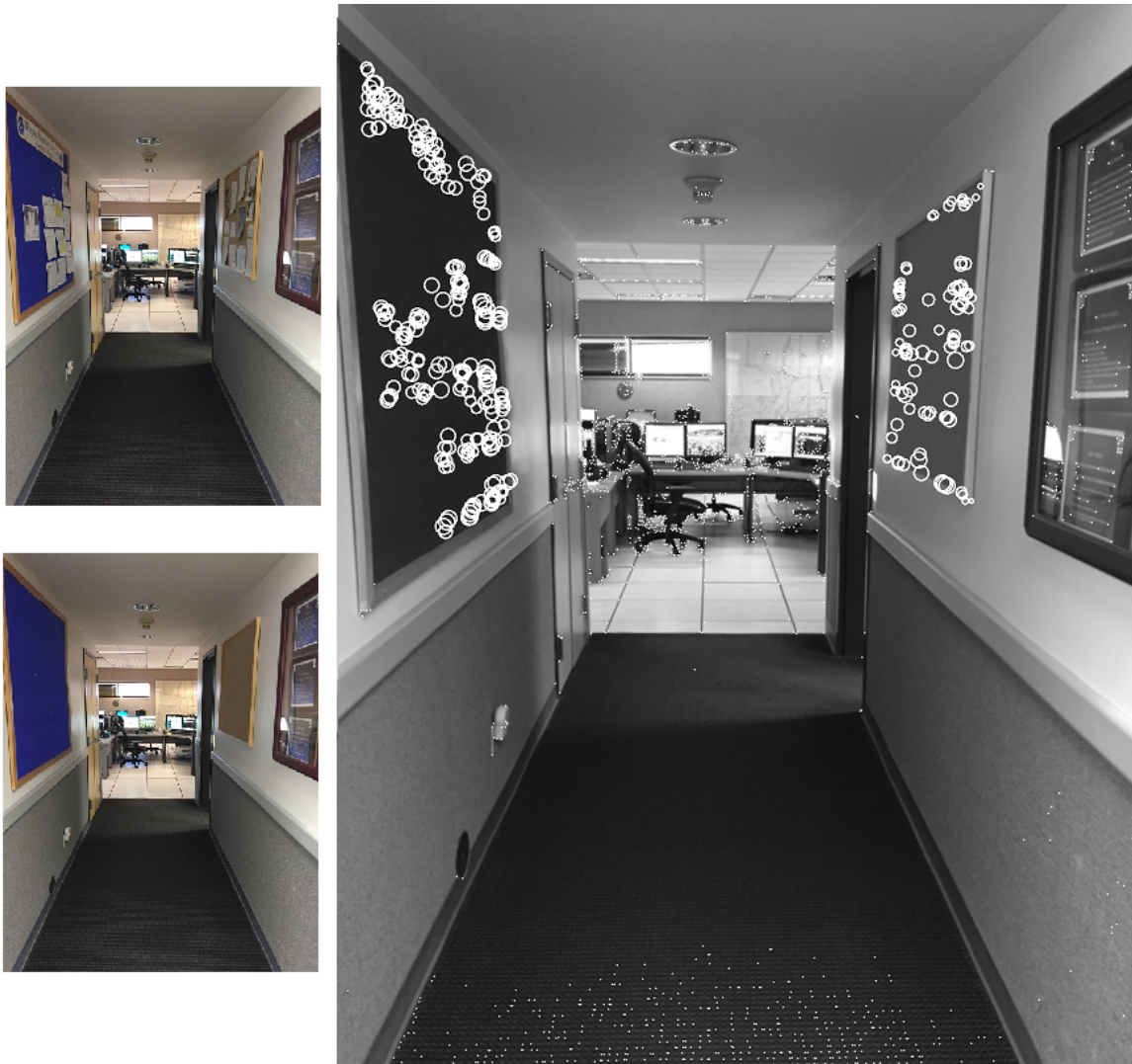
Figure 4.3: Keypoint distance change detection method showed on indoor environment picture. The source and target images are shown in the left column.
