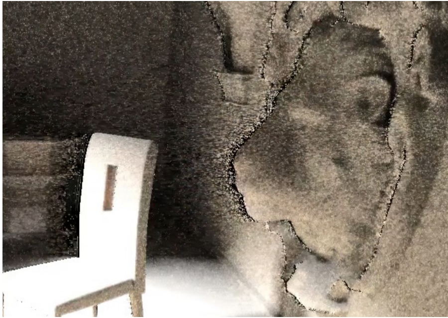
Figure 4.5: Some pixels weren't visible in previous frame and it isn't possible to blend them with a previous frame. This creates visible artifacts in the accumulation: there are some places along edges with visibly less accumulated samples. This additional noise gets filtered by our spatial bilateral filter during the next algorithm stage 4.1.4.
