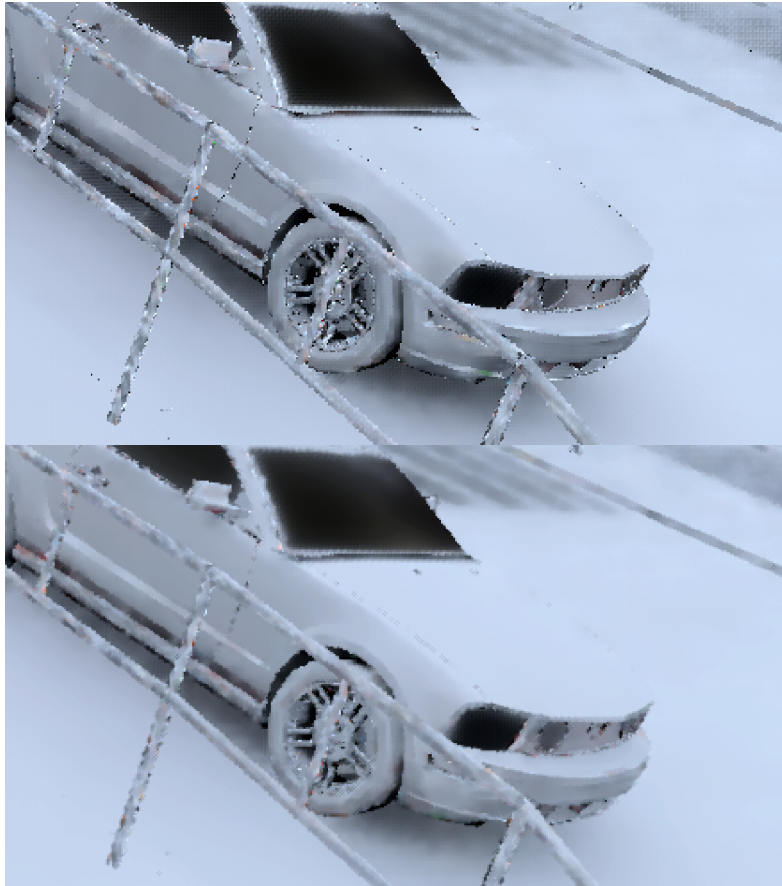
Figure 4.14: Temporal antialiasing smooths both jagged lines (easily visible with complex geometry) and noisy low-sampled areas (like the han rail here). Top image is without temporal antialiasing, bottom one with it.
