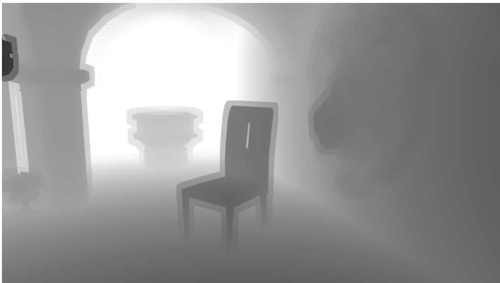
Figure 4.20: Illustration of a eroded depth buffer: all holes with incorrect surfaces (much further compared to the eroded depth buffer) get rejected.
