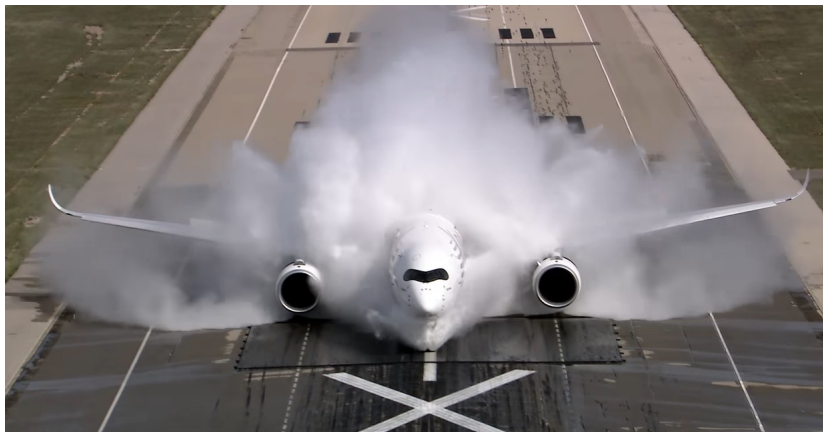
Figure 1.2: Airbus A350 XWB during a water ignition test. This test is held to confirm the aircraft ability to operate safely in wet conditions, i.e., engines will not go off in a heavy rain. Credits: Airbus 2
