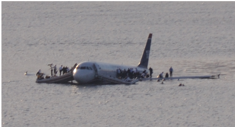
Figure 1.5: US Airways flight 1549 after an emergency landing on the Hudson River. This Airbus A320 had to land on a river in the middle of New York after a collision with a flock of Canada geese causing almost the total loss of thrust. Credits: Wikipedia 5
