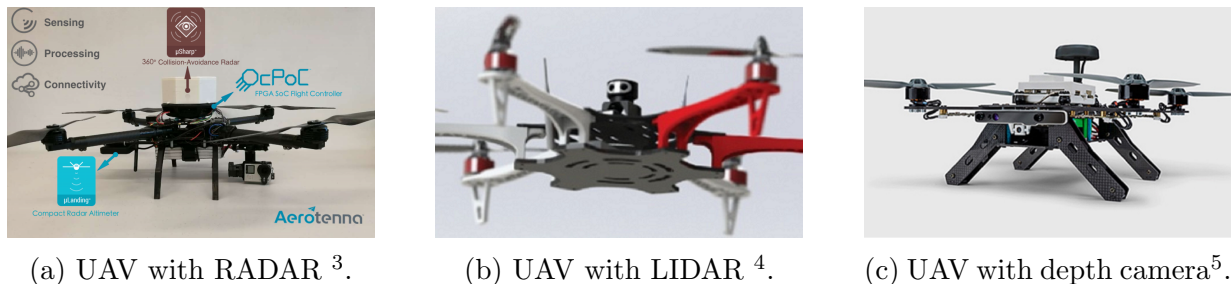
Figure 2: Examples of using sensors for detection of obstacles mounted on UAVs.
