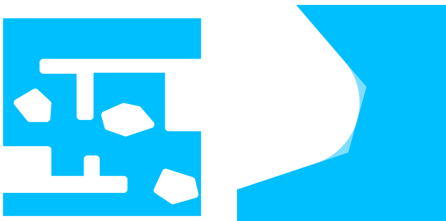
Figure 6.2: \mathcal{W} generated with both round and square joint type. The first one is drawn in lighter shade of blue overlapped by the second one in richer color. Left: the whole picture. Right: detail.
