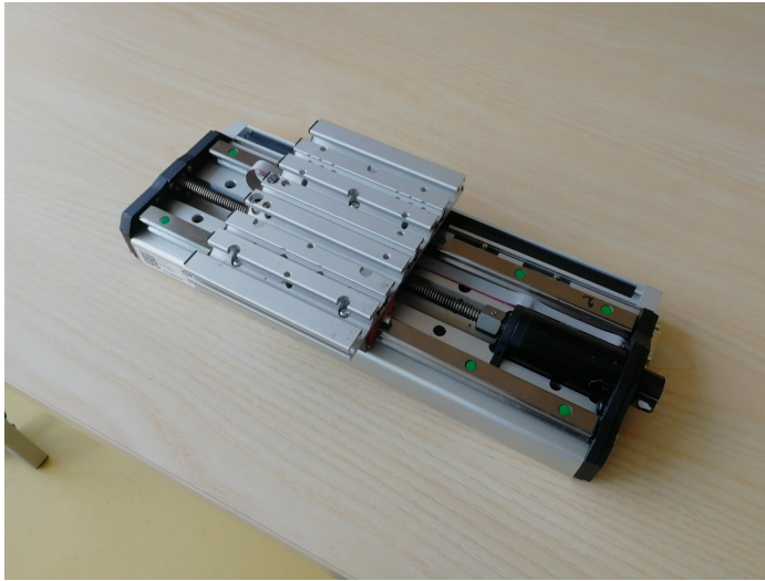
Figure 4.11: Device, which allowed accurate changes in the sphere's position.
