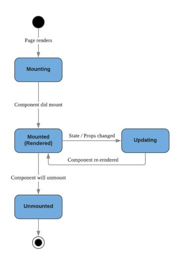
Figure 2.1: State diagram of React Component Lifecycle
