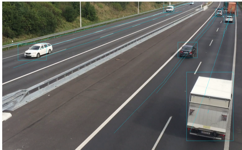
Figure 2.1: Tracking objects in one camera. The rectangles are detection of the objects. The lines are the identified tracks of the objects across multiple frames.
